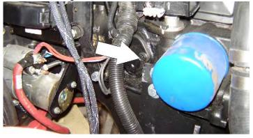
Lube Point(s) - Fill Cap/Spin-on Element (JLG P/N 7027965) Capacity - 4.5 qt. (4.25 L) w/filter Lube - EO Interval - 3 Months or 150 hours of operation Comments - Check level daily/Change in accordance with engine manual. 10. Fuel Filter - Deutz D2011
