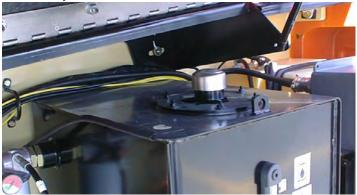
Lube Point(s) - Fill Cap Capacity - 40 gallons (151 L) Tank; 77 gallons (291.4 L) System Lube - HO Interval - Check Level daily; Change every 2 years or 1200 hours of operation.
