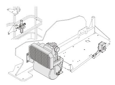
SkyAir<sup>™</sup> supplies compressed air to the platform. A filter/regulator located in the platform controls air pressure. The on/off switch is located in the engine compartment. This accessory receives power from the SkyPower<sup>™</sup> system.
