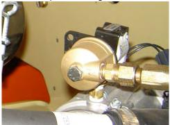
Interval - 3 Months or 150 hours of operation Comments - Replace filter. Refer to Section 7.5, Propane Fuel Filter Replacement
