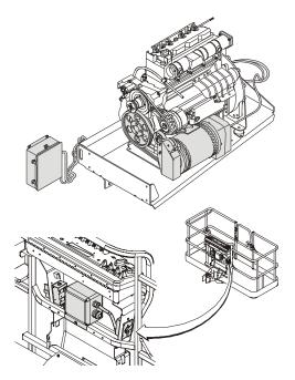
The SkyPower<sup>™</sup> system supplies AC power to the platform through an AC receptacle to run tools, lights, cutting, and welding equipment.
