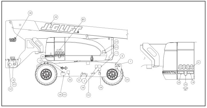
Figure 4-9. Decal Installation - Sheet 1 of 5
