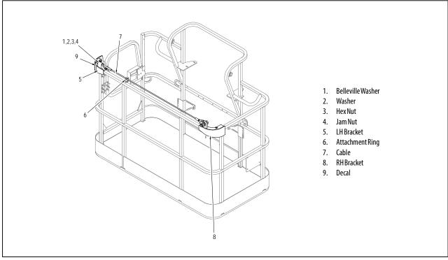
Figure 6-2. Bolt-On External Fall Arrest System
