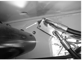
Figure 2-5. Tower Boom Vertical Limit Switch
