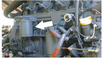
Lube Point(s) - Fill Cap/Spin-on Element Capacity - 11 Quarts(10.5 L) Crankcase Lube - EO Interval - Every Year or 1200 hours of operation Comments - Check level daily/Change in accordance with engine manual.
