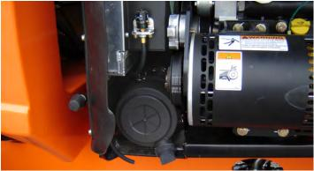
Lube Point(s) - Replaceable Element Interval - Every 6 months or 300 hours of operation or as indicated by the condition indicator **13.** Fuel Filter (Propane) - GM Engine
