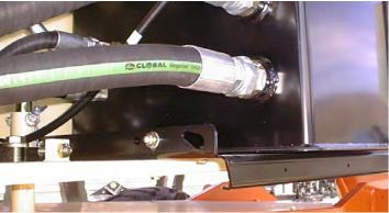
Lube Point(s) - 2 Grease Fittings Capacity - A/R Lube - MPG Interval - Every 3 months or 150 hrs of operation Comments - Remote Access 2. Wheel Bearings
