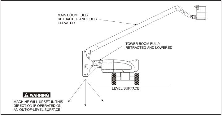
Figure 4-2. Positions of Least Backward Stability (Sheet 1 of 2)
