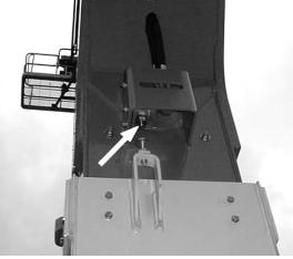
Figure 2-6. Tower Boom Horizontal Limit Switch
