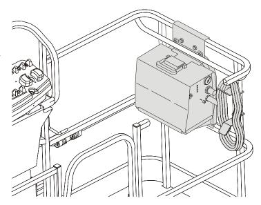
SkyCutter<sup>™</sup> is capable of cutting up to a thickness of 3/8" metal. It can produce 27 A at 92 VDC at 35% duty cycle or 14 A at 92 VDC at 60% duty cycle. It receives power from the SkyPower<sup>™</sup> system.
