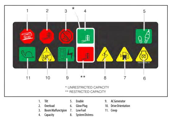
Figure 3-5. Platform Console Indicator Panel
