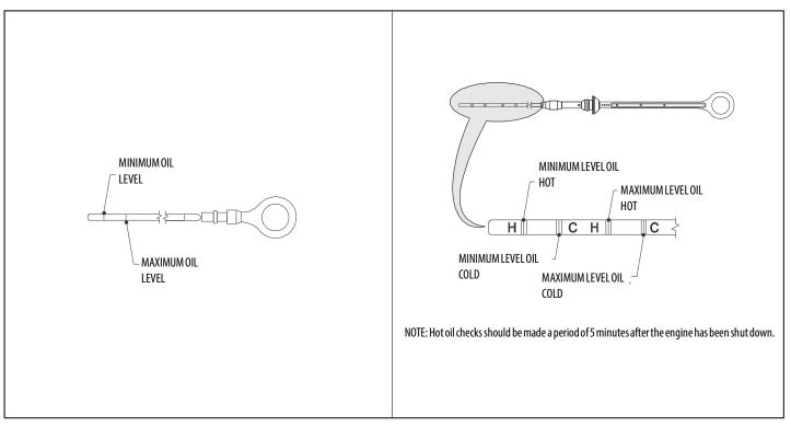
Figure 7-6. Deutz 2011 Engine Dipstick
