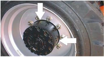
Lube Point(s) - Level/Fill Plug Capacity - 17 oz. (0.5 L) - 1/2 Full Lube - EPGL
