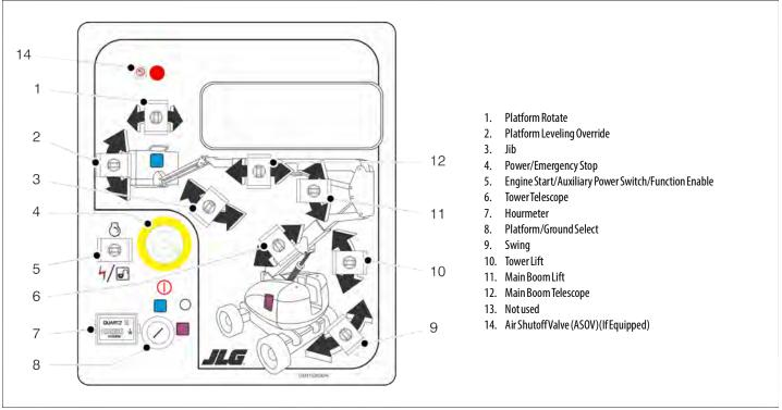
Figure 3-1. Ground Control Console
