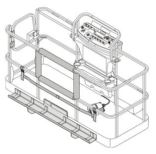
SkyGlazier<sup>™</sup> allows glaziers to position panels efficiently. The glazier package consists of a tray that attaches the bottom of the platform. The panel rests on the tray and against top-rail of the platform, which is padded to prevent damage. SkyGlazier<sup>™</sup> includes a strap to secure the panel to the platform rail.
