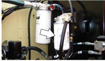
Lube Point(s) - Replaceable Element Interval - Change in accordance with engine manual
