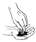
Lube Point(s) - Repack Capacity - A/R Lube - MPG Interval - Every 2 years or 1200 hours of operation 3. Wheel Drive Hub
